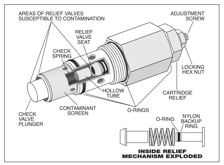
**E Series** complete assembly part number: PE-1231V, PE1-1231V **S Series** complete assembly part number: PS-1231V, PS1-1231V
